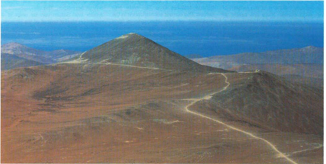
Figure 2: Paranal stands isolated and has the shape of a cone, two features of vital importance for the air flow over and around the mountain.
