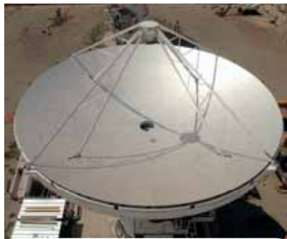
The European antenna prototype for ALMA
