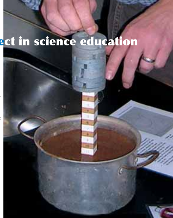
A teacher demonstrates how to measure pressure in the sand container
