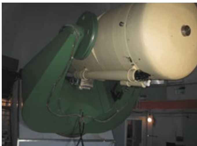
Figure 1. The 1.0-metre ESO Schmidt telescope inside the dome. The QUEST camera is inside the telescope mounted at the prime focus. The camera electronics are visible on the underside of the telescope tube with cabling running up the yoke and around the declination axis.
