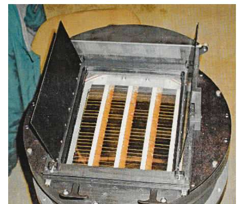
Figure 3. The 10-square-degree QUEST camera. The focal plane of the 161-megapixel camera consists of 112 CCD devices arranged in four rows with 28 CCDs each. The array spans 3.6 \times 4.6 degrees with an active area of 9.6 square degrees.
