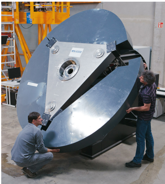
Figure 4. The electro-mechanical M5 prototype. In the centre is a dummy mirror that is moved in tip-tilt by three heavy-duty actuators mounted behind the system. The covers being installed by Pablo Barriga and Marin Dimmler give the full dimensions of the M5 mirror as it will be installed in the telescope.
