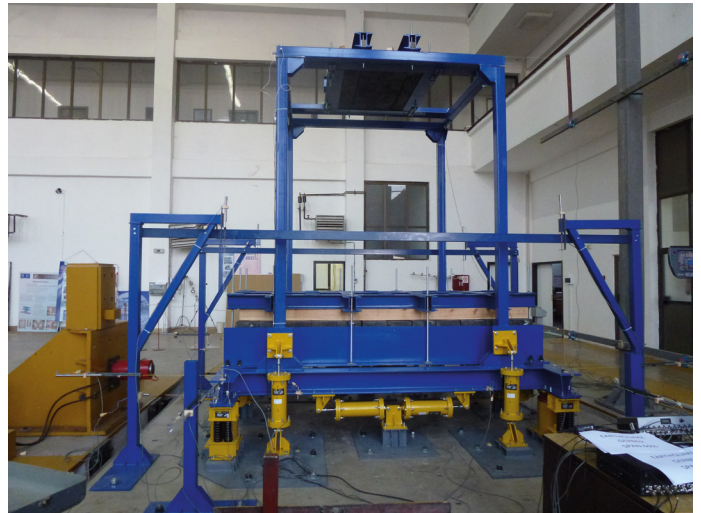
Figure 2. The seismic isolation test bed. Both the lateral and the vertical components of the earthquake acceleration are significantly diminished through this isolation device.
