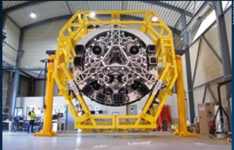
Testing of the ELT M2 mirror cell.
