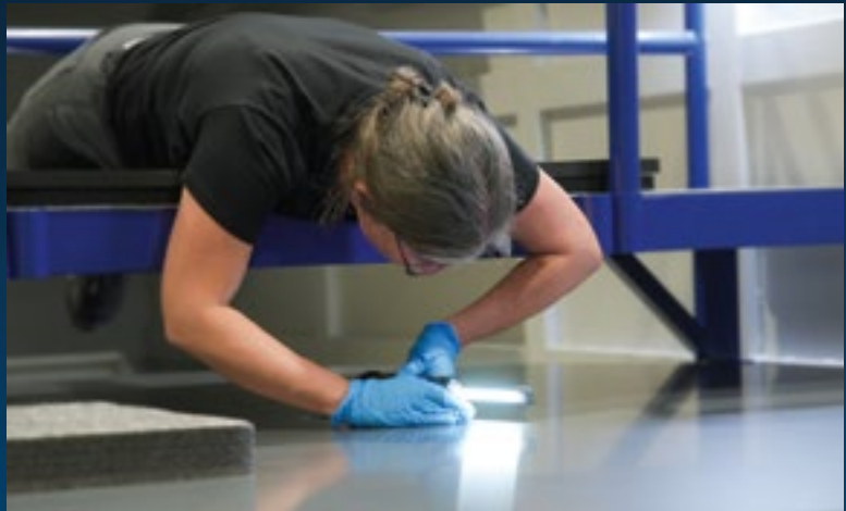
Inspecting the ELT M5 mirror blank.
