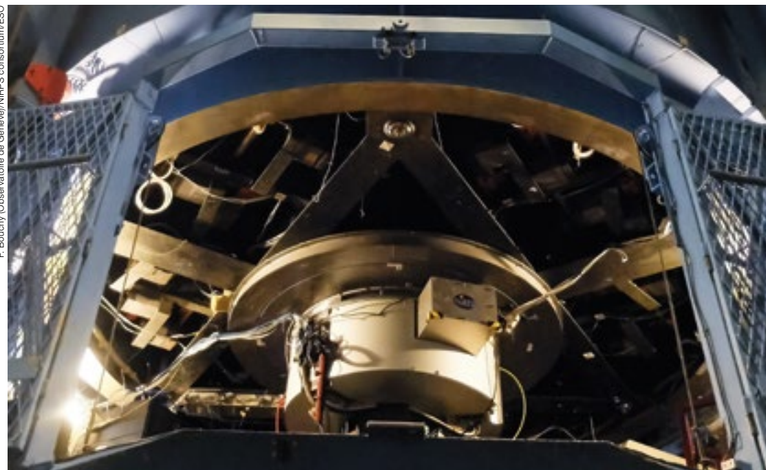
The front end of the NIRPS (Near Infra-red Planet Searcher) instrument, including its adaptive optics system, sits just under the primary mirror of ESO's 3.6-metre telescope.
