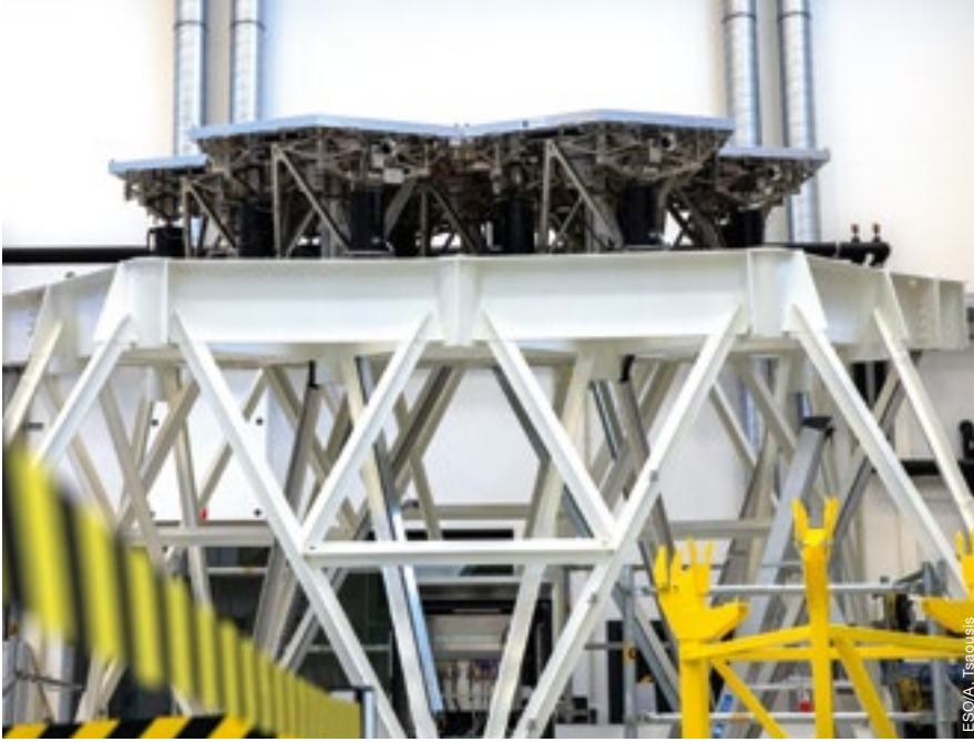
Above: Testing of ELT M1 segment supports at the ESO Headquarters.
