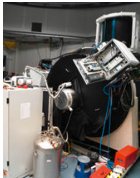
The AOF test configuration in the Garching laboratory: the deformable secondary mirror sits on top of the ASSIST bench and the GRAAL module is mounted on the Nasmyth focus simulator, with the CAMCAO silver cryostat in the foreground.
