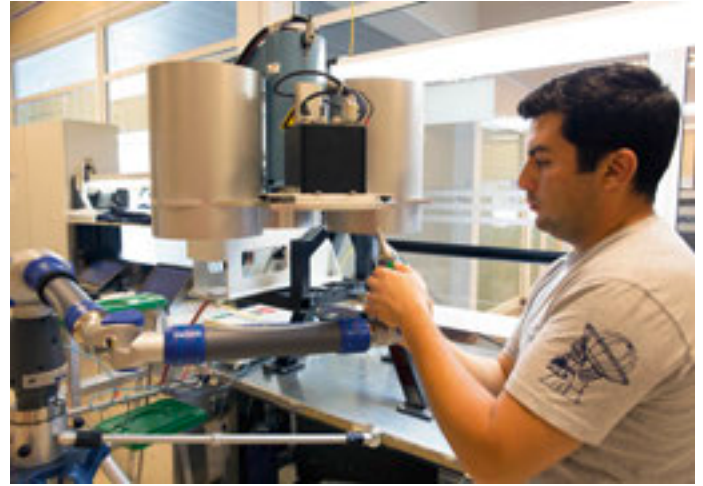
An amplitude calibration device being serviced at the OSF. Each ALMA antenna has one of these devices to calibrate the radio signals.
