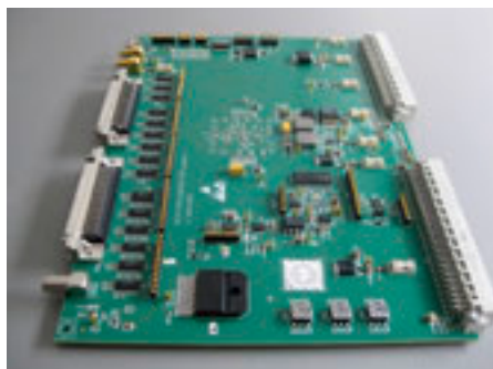
Replacement avalanche photodiode board for NACO, based on field-programmable gate array technologies.
