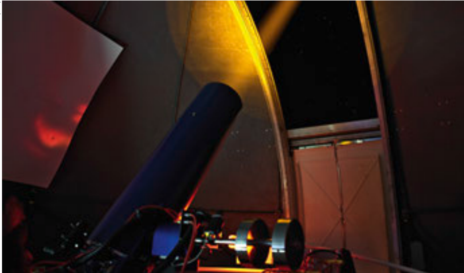
The laser launch telescope for the ESO Wendelstein laser guide star unit under demonstration at the Teide Observatory.
