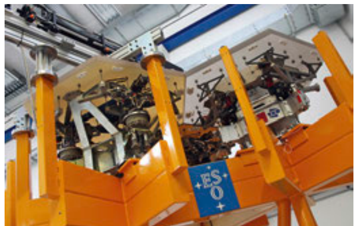
Two test segments for the E-ELT 39-metre primary mirror. The prototype support system on the left was produced by CESA (Spain) and the one on the right by VDL/TNO (the Netherlands).
