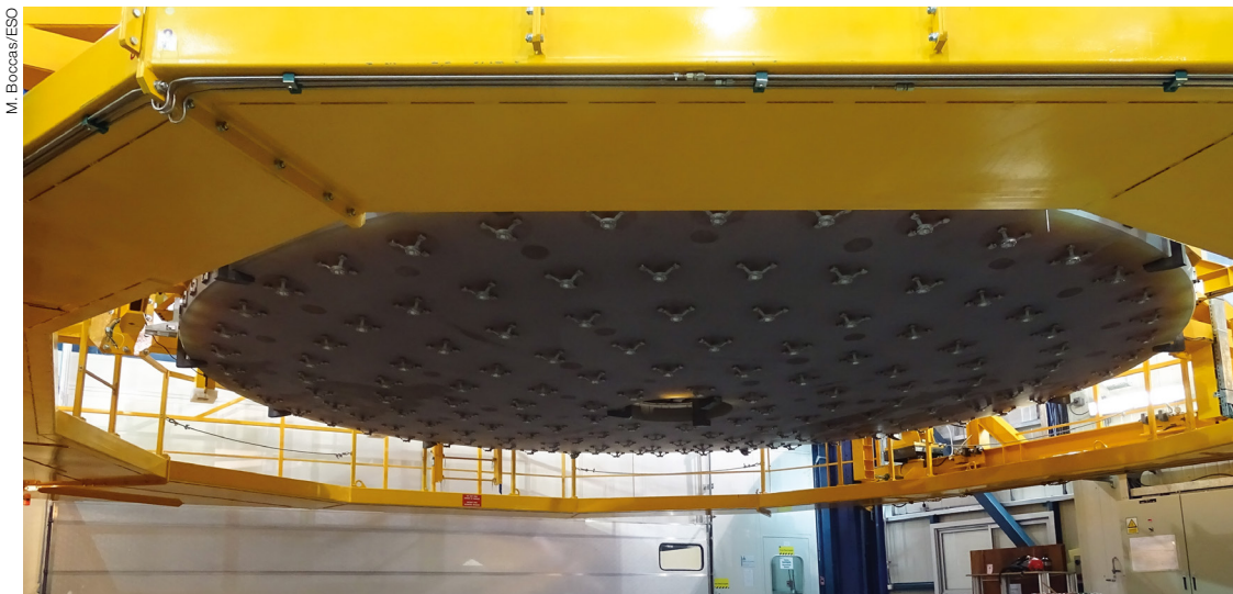
The VLT M1 Mirror Handling Tool is used to move the VLT's 23-tonne, 8.2-metre-diameter primary mirrors when they need to be recoated.
