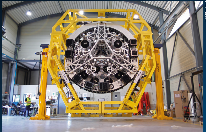
Testing of the ELT M2 mirror cell.
