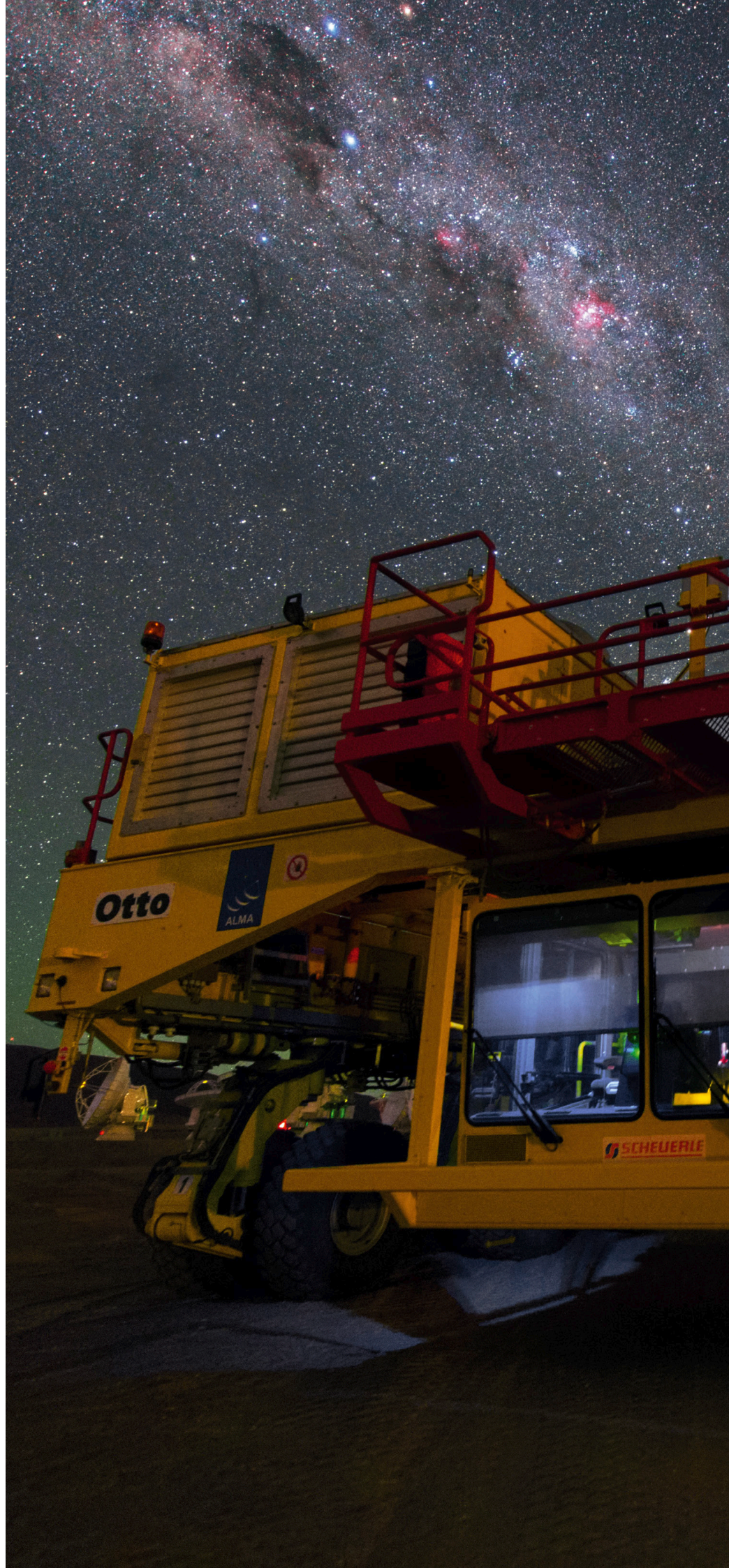
This picture shows the ALMA transporter Otto. It is one of two transporters which are able to carry the huge antennas up to the Chajnantor Plateau and move them around there.
