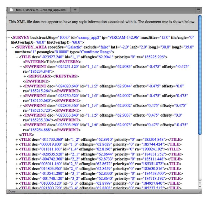
Within the <Pawprint /> element the 'id' is constructed as *Tile\_ID:PawprintNumber*.
