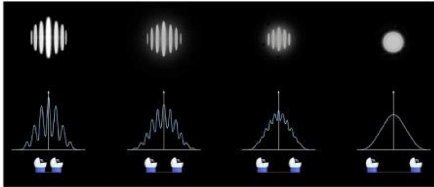
Interferometric Fringes at Different Telescope Baselines
