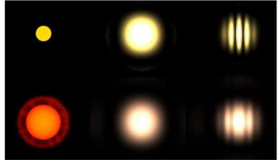
Interferometric Fringes from Star with Different Angular Diameters
