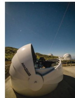
Fig. 1 | The GOTO project is an array of telescopes on custom mounts inside clamshell domes at the Roque de los Muchachos Observatory in La Palma, Spain. It aims to find visible counterparts to gravitational wave-generating merger events. Credit: K. Ulaczyk/University of Warwick
