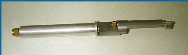
Positioning unit with 2 step motors
