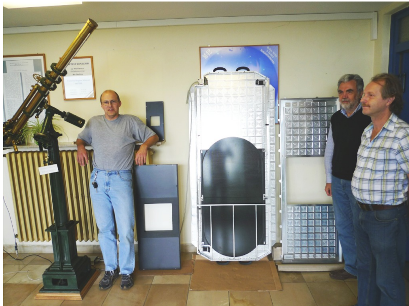
Figure 1. A collection of shutters of various sizes and at various stages of completion together with the authors (from left: Martin Polder, Klaus Reif, Philipp Müller). The smallest shutter (top left) is 100mm, below 280mm. The door size shutter in the center is for Decam. It has a circular aperture of 600mm. At the right hand side is the base plate of a new Pan-STARRS shutter with its 480mm aperture.
