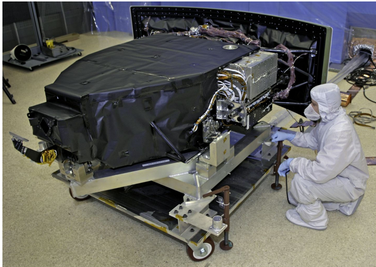
Fig. 1. Wide Field Camera 3 in environmental testing at Goddard Space Flight Center in 2008.
