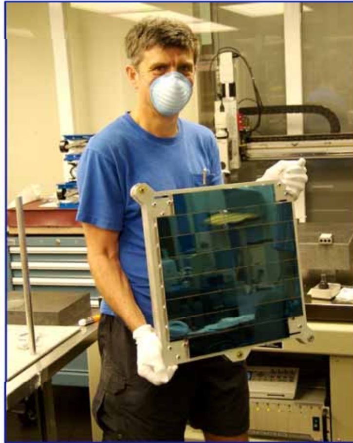
60 Orthogonal-Transfer CCDs Pan-STARRs (3° WFOV) 1.36 Gpixels
