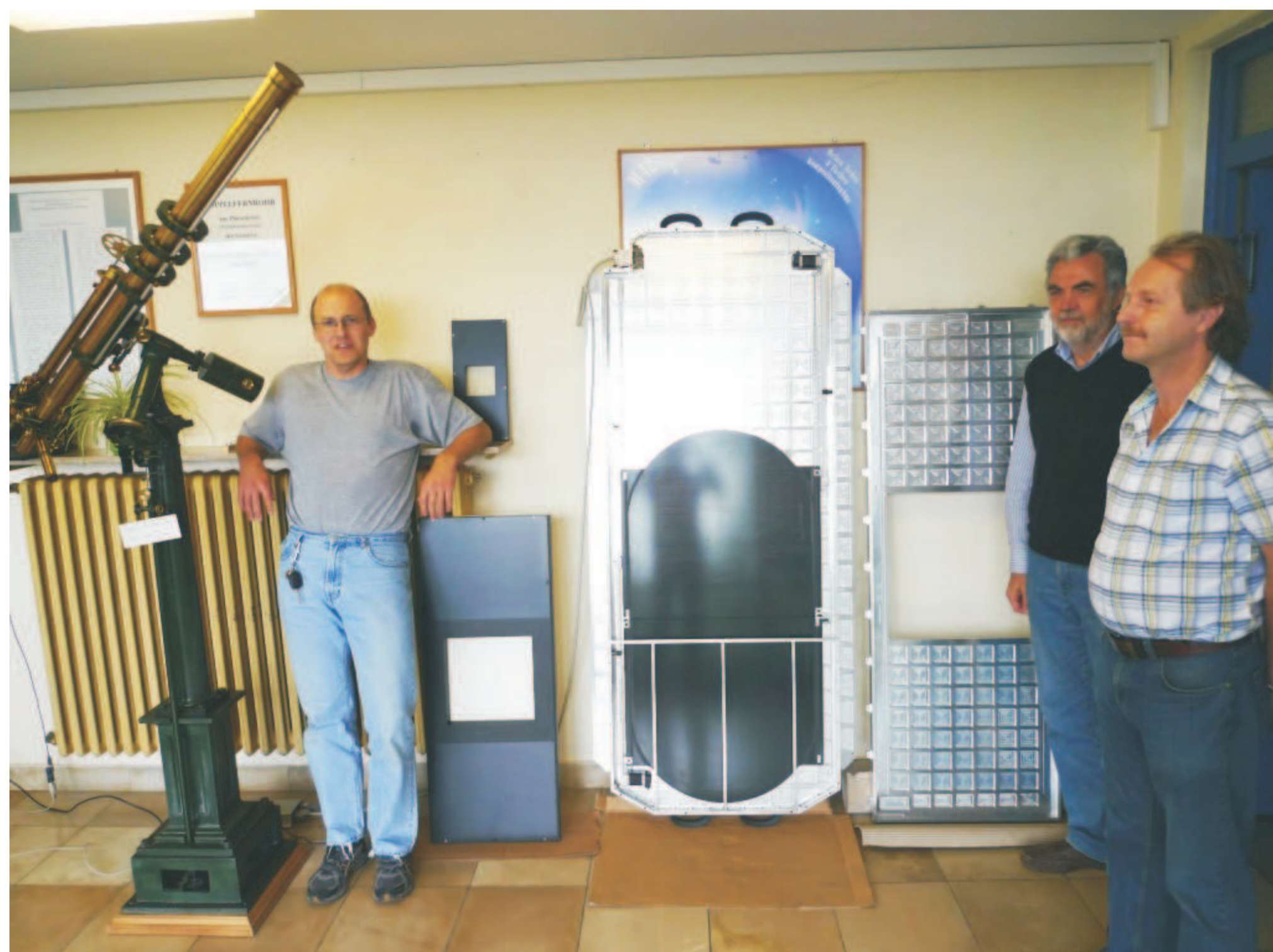
A collection of shutters of various sizes and at various stages of completion together with the authors (from left: Martin Polder, Klaus Reif, Philipp Müller). The smallest shutter (top left) is 100mm, below 280mm. The door size shutter in the center is for Decam. It has a circular aperture of 600mm. At the right hand side is the base plate of a new Pan-STARRS shutter with its 480mm aperture..
