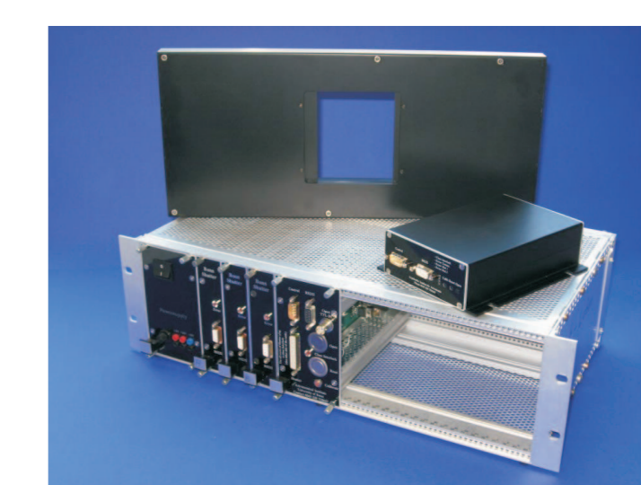
100mm shutter with old and new electronics
