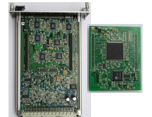
Digital pattern generation module realized as piggyback board.
