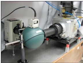
Optical test equipment One of 3 complete test setups. 3 CCDs can be tested in parallel.
