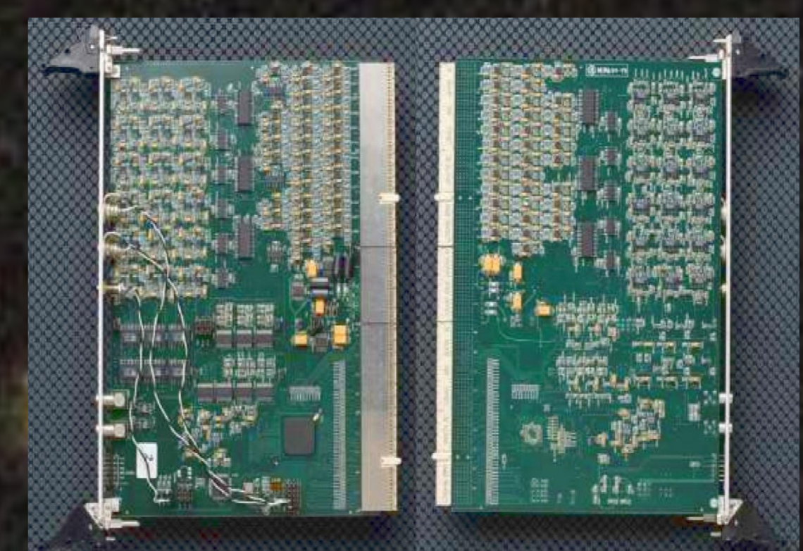
Electronics boards based on the Monsoon read-out system developed by NOAO
