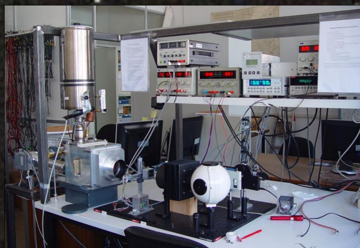
Set-up testing station for CCD characterization
