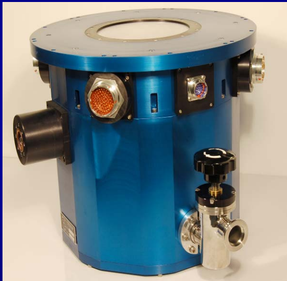
Dewar 61 Pin I/O and 18 Pin Temp Connectors
