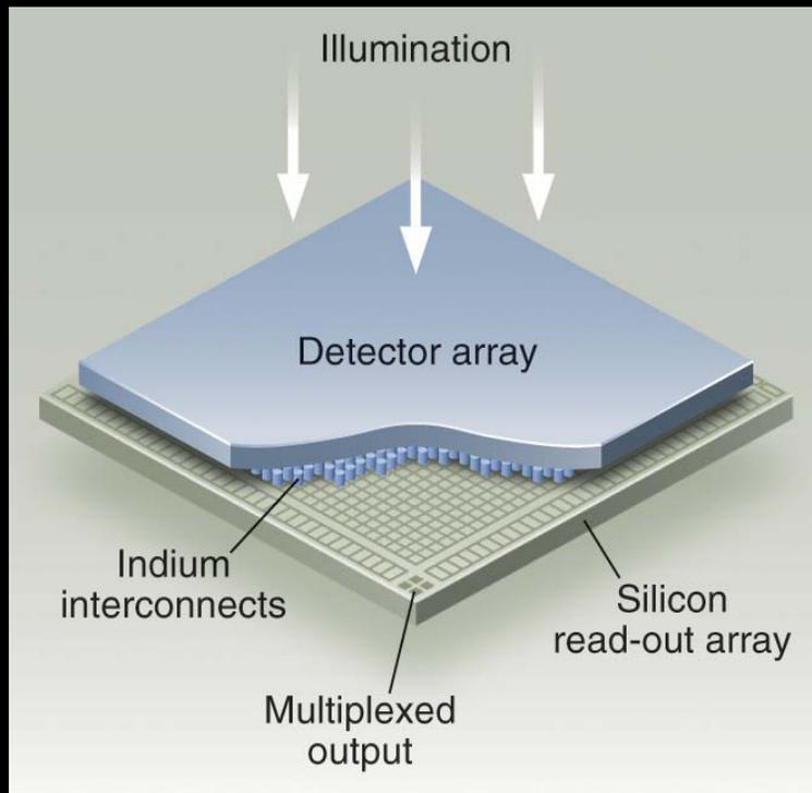
**The functionality of a Readout Integrated Circuit (ROIC) is only limited by:**
