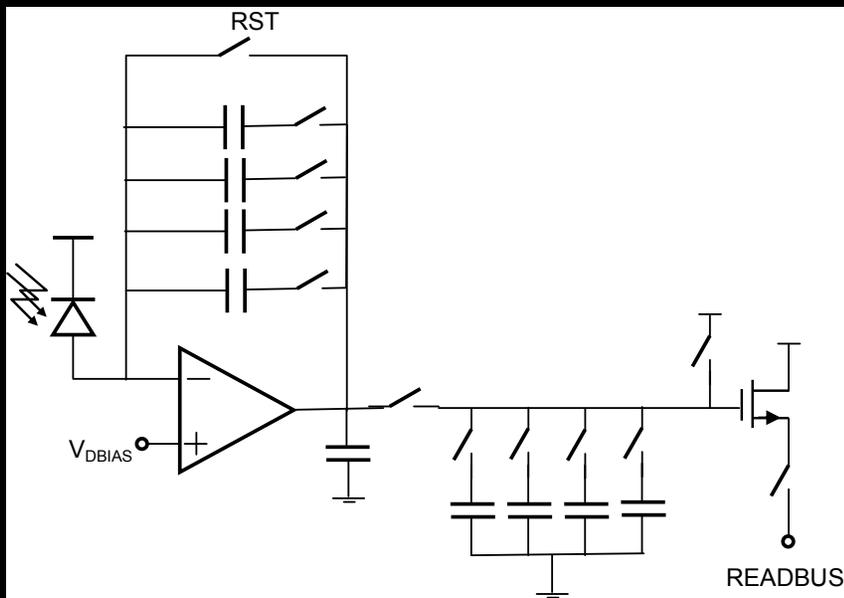
Teledyne has made a sensor that takes three successive 280 nsec exposures, using charge caching approach similar to what is shown in schematic at left.
