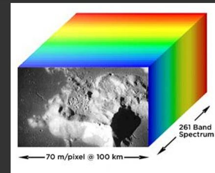
Moon Mineralogy Mapper resolves visible and infrared to 10 nm spectral resolution, 70 m spatial resolution
