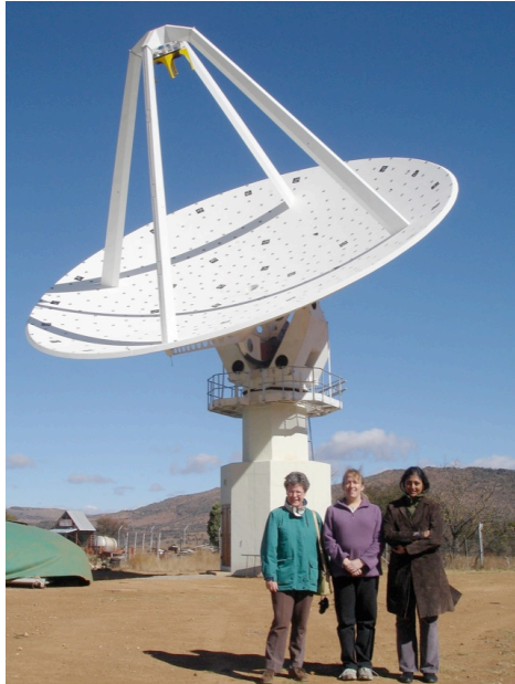
ZA: 15 m fibreglass+foam dish (<2mm r.m.s.)
