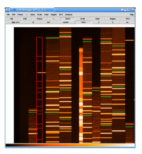
Often a global shift is not enough, and a detailed adjustment of individual slits becomes necessary: here we reposition individual arc lamp lines one by one
