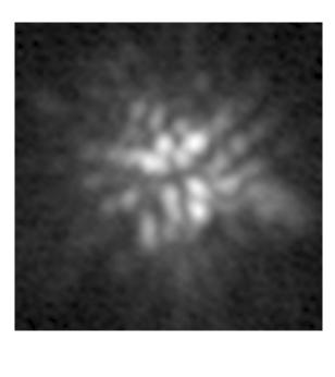
One typical speckle interferogram of NGC 1068 taken through a K-band filter at the Russian 6 m telescope. NICMOS 3 array. Exposure time 200 ms. Shown field of view 1.85x1.85 arcsec.
