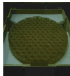
Figure 2.6 [JPG: 419k]. The first VLT M2 Beryllium Mirror in the test laboratory of DASA (Ottobrunn near Munich, Germany), during the determination of its inertia and center of gravity. The mirror is covered by a peelable protective layer. (September 1997).
