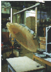
Figure 3.10 [GIF: 268k]. The lightweighted M3 mirror.
