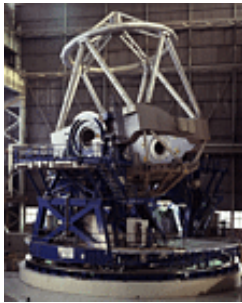
Figure 2.1 [JPG: 128k]. Mechanical structure of UT4 during pre-assembly at Ansaldo (Milan, Italy).
