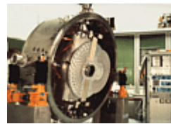
Figure 8.14 [GIF: 144k]. ISAAC, almost completely assembled with the large slit/mask wheel clearly visible at the front.
