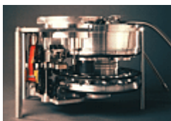
Figure 8.16 [GIF: 120k]. One ISAAC camera. Visible are the objective wheel, and two filter wheels. The detector is not shown.
