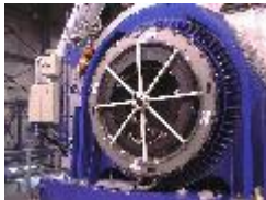
Figure 3.20 [JPG: 176k]. The Nasmyth Adapter/Rotator, installed at the UT1 (March 1998).
