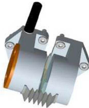
Figure 16: Conceptual design of the Mk II Heidenhain optical sensor. The two halves contain, respectively the reticle and scale and are mounted to adjacent mirror segments. A light-tight bellows would surround the gap between the two halves.
