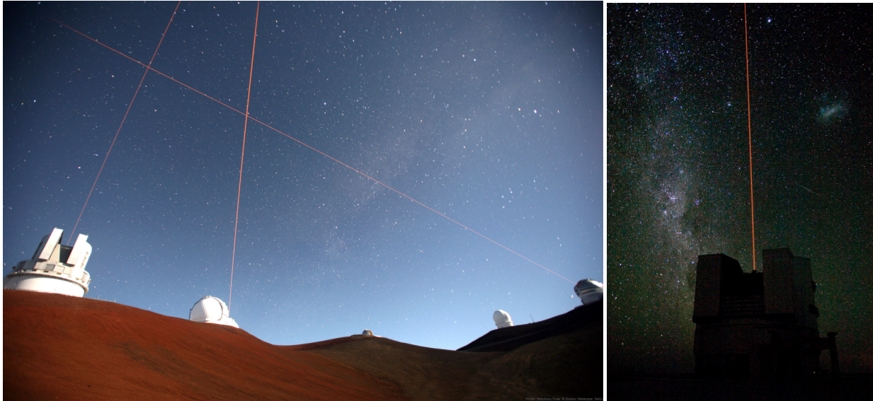
Figure 1: (left) Three lasers operating on Mauna Kea, From left to right, Gemini, Subaru and Keck II (Photo: Tetsuharu Fuse, Subaru, NAOJ). (Right) Laser propagating from Yepun during first light (ESO PR Photo 0607a, credit: G. Huedepohl) .
