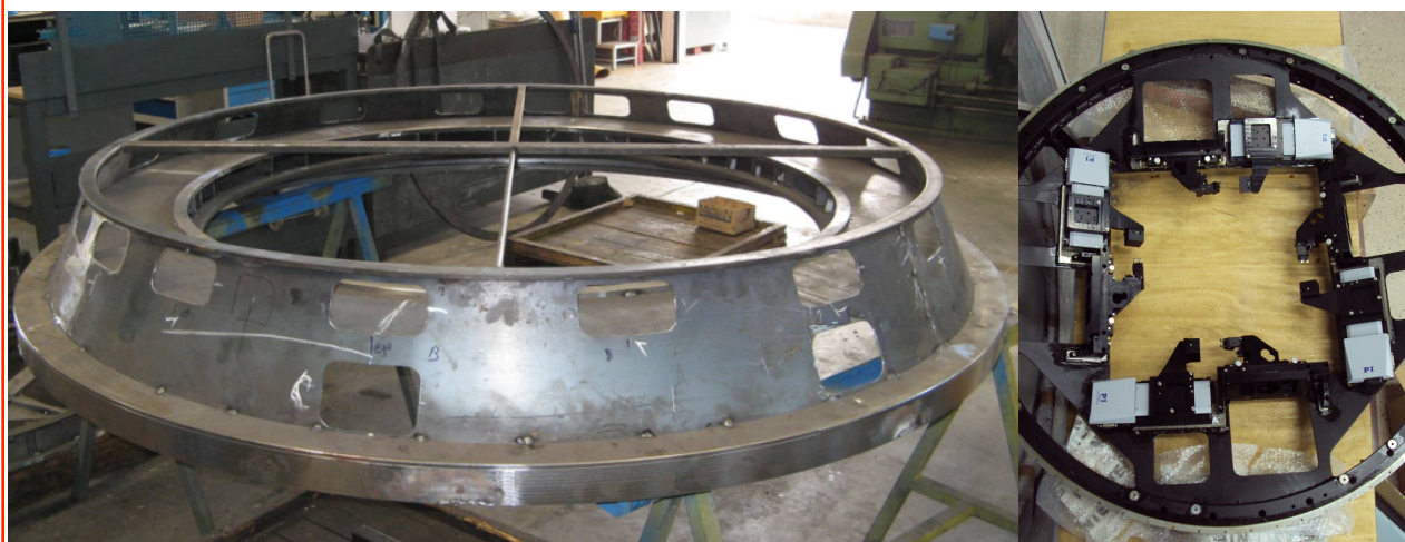
Figure 8: GRAAL Components: left, the main structure that will replace the spacer between the Nasmyth A/R and the Hawk-I instrument; it will contain all opto-mechanical components. Right: the WFS assembly pick-up arms with PI linear stages for the trombone (laser guide star focusing).
