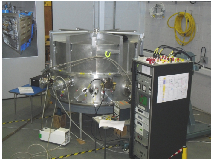
Figure 3: The KMOS main cryostat undergoing its first cooldown cycles. The closed-cycle coolers are visible around the base of the cryostat; the remaining ports contain the feedthroughs for some of the 1500 electrical connections into the cryostat. The electronics rack to the right contains all the housekeeping electronics and will eventually be mounted on the Nasmyth platform.
