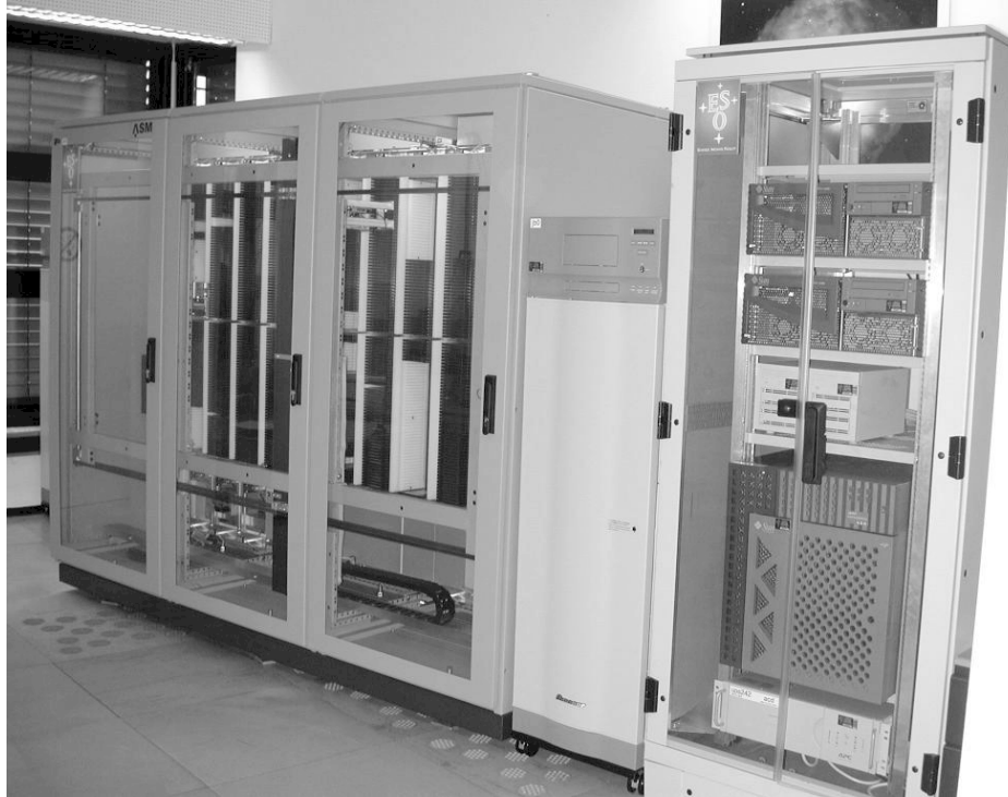
Fig. 1. This figure shows the scientific online archive in the Archive Operations Room in 2002. The DVD jukebox with its 1087 slots and 6 DVD readers on the left, another type of DVD jukeboxes with 670 slots and 4 DVD readers in the middle as well as the computer system with 4 external disks hosting the DSS, GSC and USNOA catalogs. All components were supplied through a single 3 KW Uninterruptible Power Supply on the bottom of the rack.
