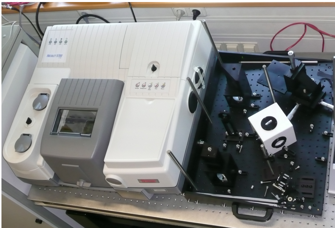
Figure 7: Commercial Fourier Transform Spectrometer in the ESO IR laboratory. On the right hand side part of the optical train of the FTS is replicated feeding the light from various sources to the external port of the FTS.
