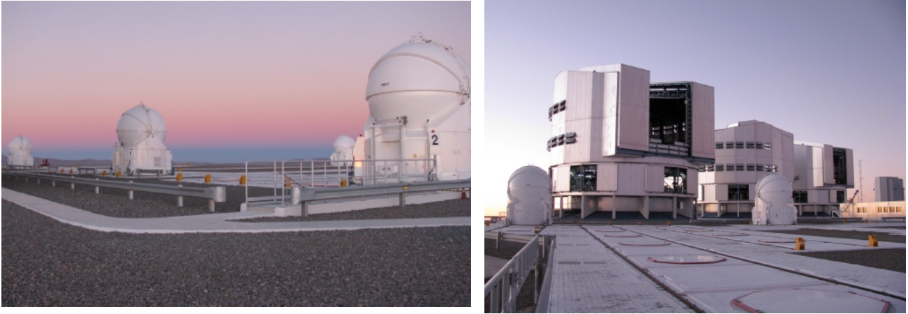
Fig. 1. The VLT Interferometer at Paranal in 2008. On the left picture, one can see the four ATs spread out on the summit, offering a variety of size and orientation of baselines. On the right picture, one can see two of the ATs in front of the UTs. In the foreground, some of the ATs stations are visible with their covers.
