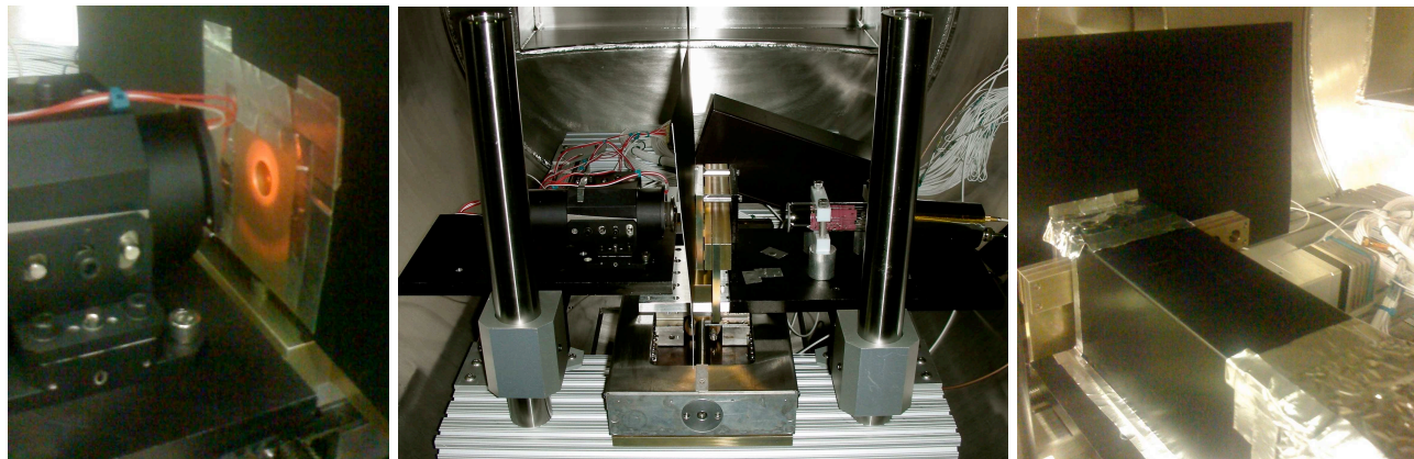
Figure 3. Vacuum lamp-test setup. Left panel shows an end-of-life lamp illuminating the fixed aperture block. Center panel shows a side view of the linear stage and the exposed PMT on the right. Right panel shows the test configuration of the PMT. Filter holes on the stage can be seen in the middle of the image just to the right of the PMT housing.
