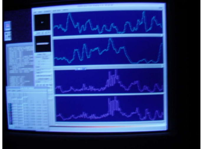
Fig. 3 – Sample of interferometric and photometric outputs, on siderostats, in open loop, during June 2003 system set-up. Performance limited by scintillation on 80 mm siderostat aperture.
