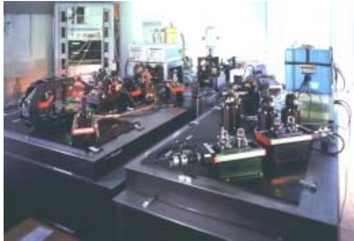
Figure 6: VINCI Beam recombining optics
