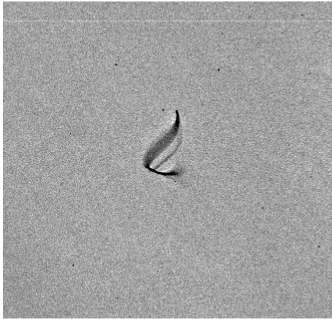
Figure 7.2-9, Dust particle, (flat field exposure), extending over a 47x67 pixel box at X=1922,Y= 905.
