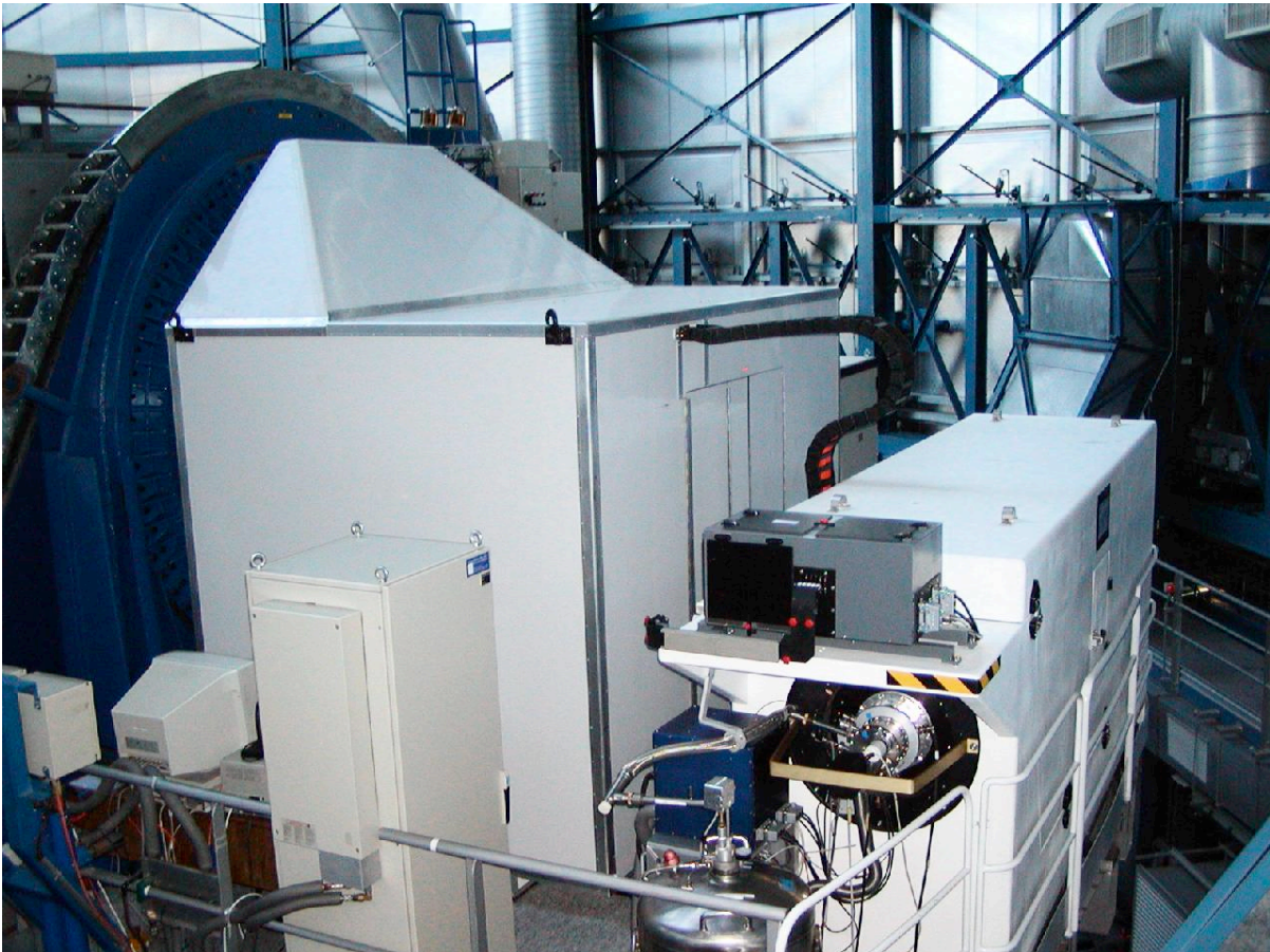
Figure 1: FLAMES at the Kueyen VLT Nasmyth A platform. On the left is the Oz Poz enclosure, on the right the Giraffe enclosure. The Fibre trail connects the two enclosures, and the Giraffe CCD dewar and continuous nitrogen cryostat is well visible
