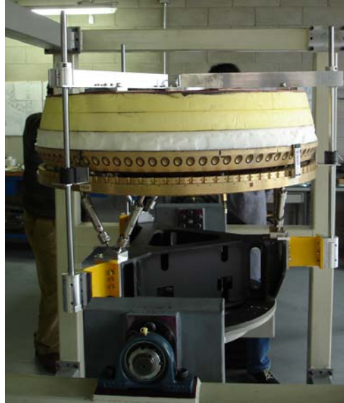
Fig.2 Left: the LBT adaptive secondary unit. Right: the unit in assembly phase. Courtesy of ADS.
