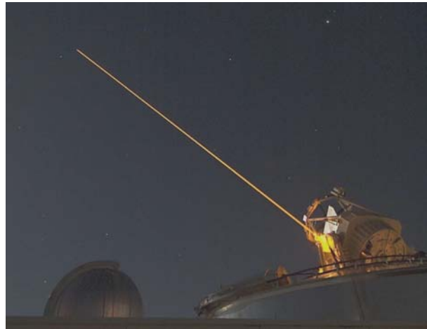
Figure 8: Starfire Optical Range. 35W of a sum-frequency laser at 589nm have been propagated to the Mesosphere
