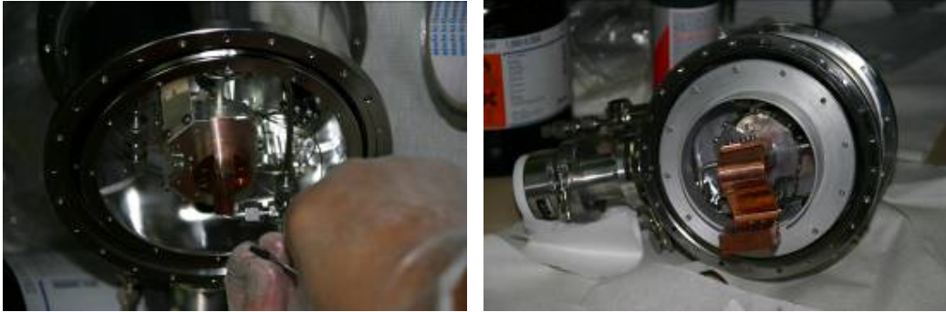
Figure 3: the modified CFC, while mounting the cold finger and the thermal straps.
