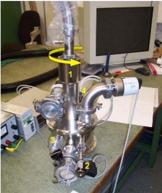
Figure 2 - the modified CFC with the new LN 2 fill port and the rotating joint (label 1).
