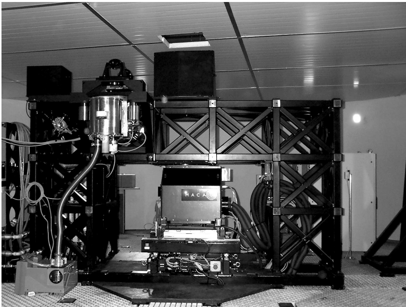
Figure 1: MACAO-VLTI on the Coude platform. The arched structure support M9, the dichroic reflecting light to the VLTI and transmitting the visible to Macao. The WFS can be seen under the arch. The shiny cryostat on the upper left is the ITC.
