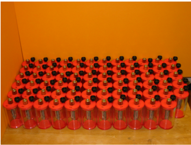
Figure 16 : Modules ready for mirror gluing
