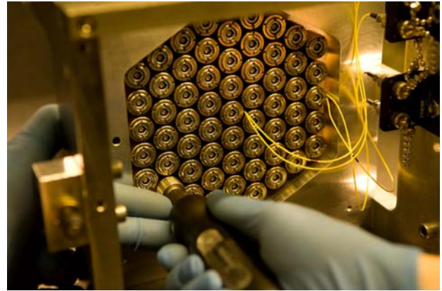
Figure 21 : Modules tightening on disk
