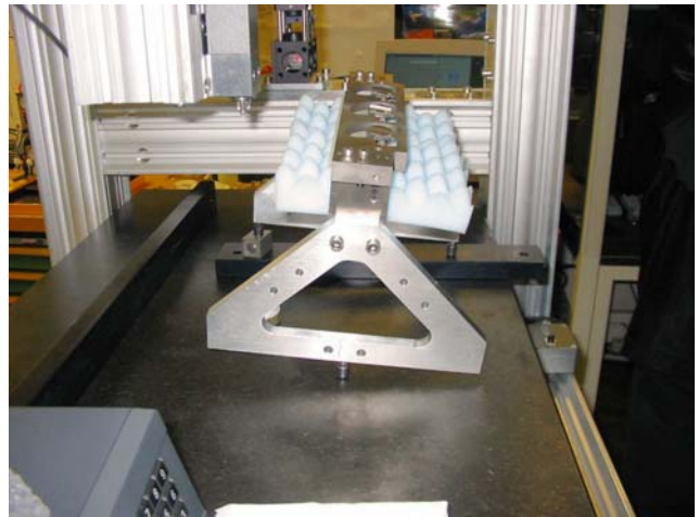
Fig. 16: Use of gravity during glue curing.
