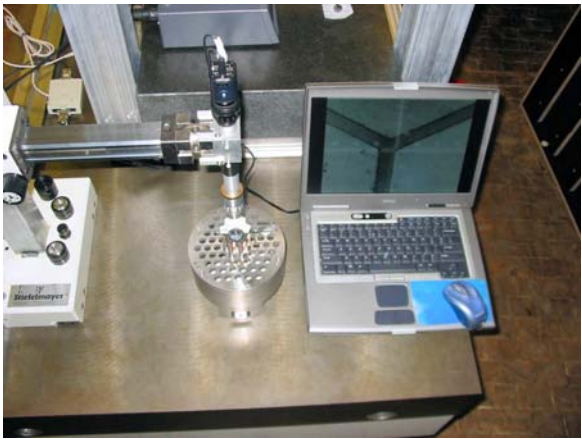
Fig. 25: Gap measurement setup
