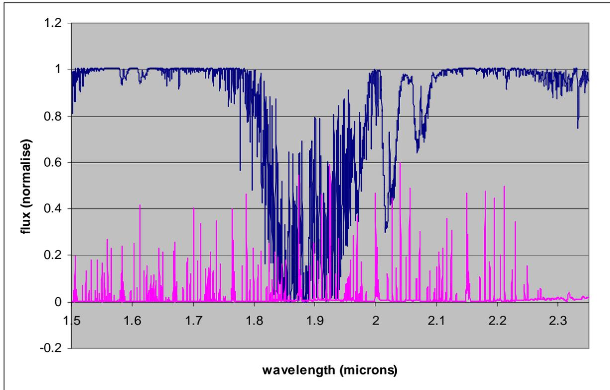
**Figure 4: Simulated transmission and OH emission spectrum for the HK grating. The OH units are arbitrary, scaled to be plotted alongside the transmission.**
