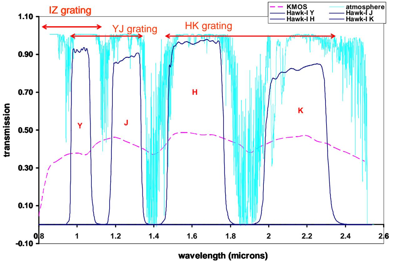
Figure 5 Hawk-I filters and KMOS wide (IZ, ZY, HK) gratings shown in red for comparison. The KMOS transmission curve includes filters and the grating efficiency curves for the original grating suite. The 0.8 $\mu$ m transmission will be improved with optimisation of the blocking before FDR. The detector QE is not included.
