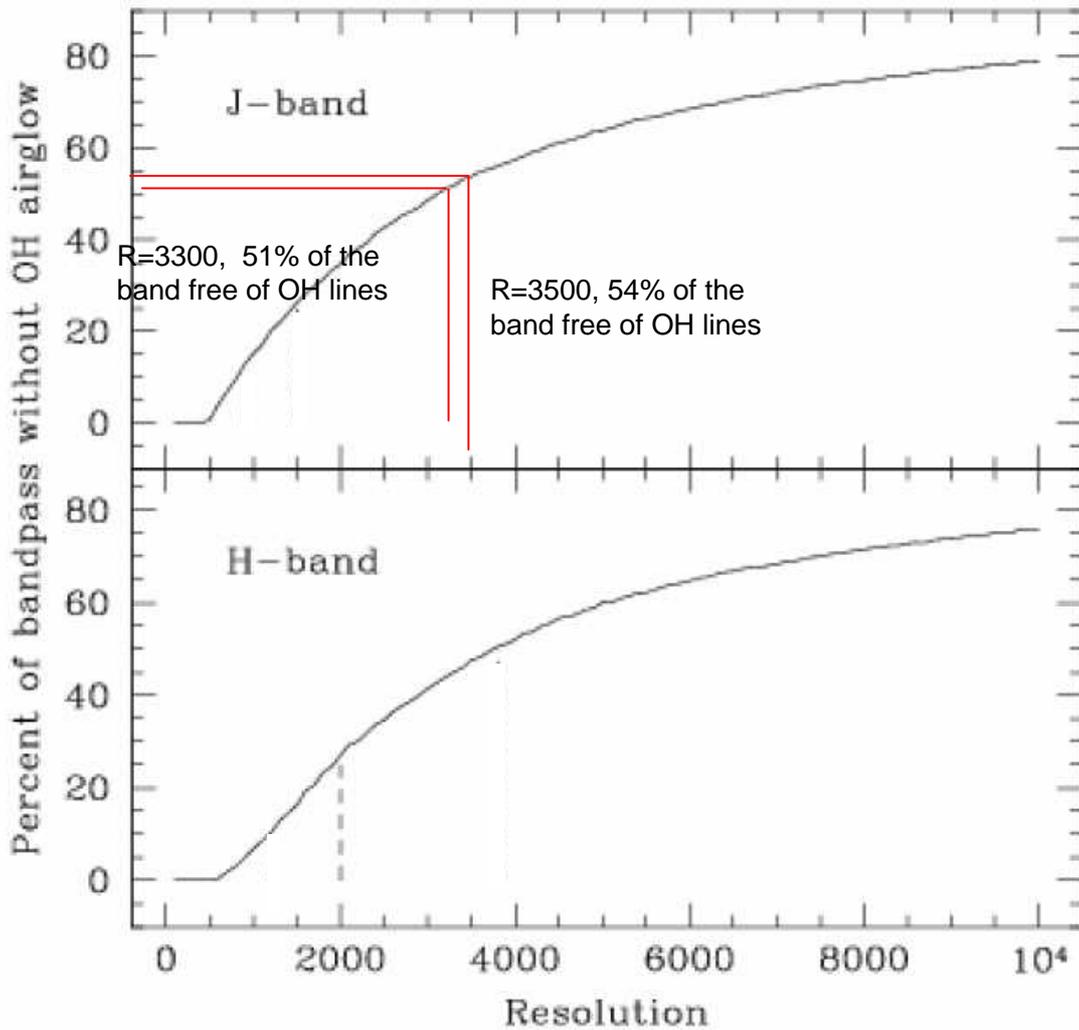
Figure 3: From Depoy & Martini, the effect of resolution on OH line coverage.
