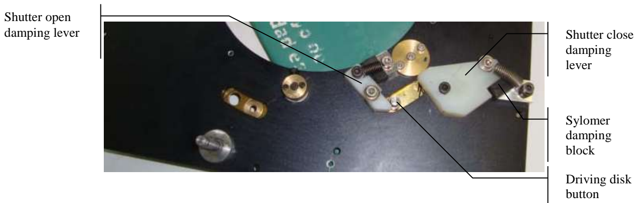
Figure 6: End of the range mechanical damping
