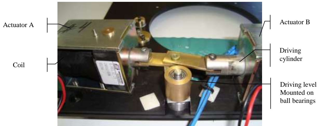
Figure 2: Electro-magnet drive system
