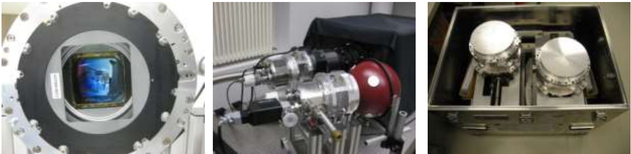
Figure 8. Left: visual inspection of detector and graded-index coated field lens window. Center: one DV mounted to spectrograph and one DV behind an integrating sphere during flat fielding. Right: ESO transport container with 2 DVs packed for shipment.
