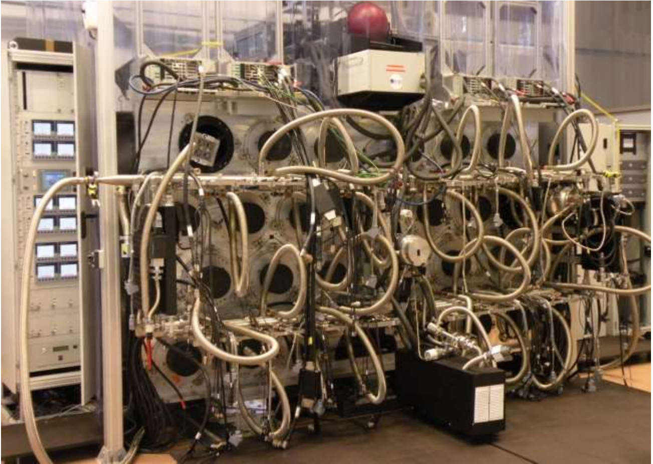
Figure 11: MUSE Vacuum Cryogenic System (with one IFU in position)
