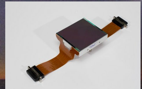
Mechanical sample of 4k x 4k e2v CCD231-84 for prototype
