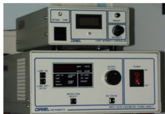
Figure 4 Halogen lamp power supply (down) and light intensity controller (up)
