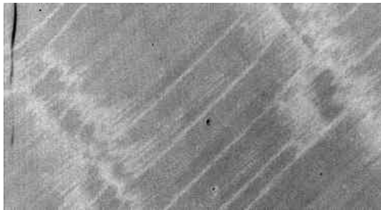
Figure 101 At 320 nm uniformity degraded by the implantation of P+ passivation layer annealed by laser after thinning)
