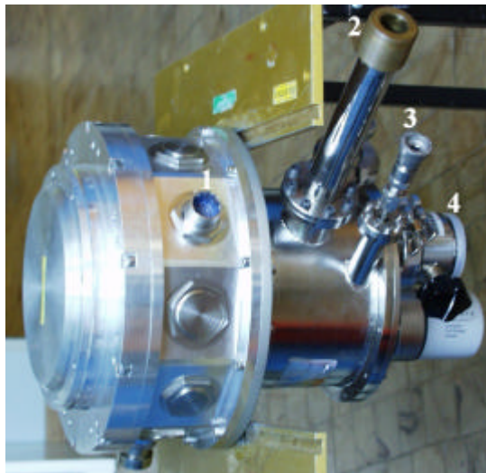
Figure 80 Detector head used on the testbench: (1) Pre-ampli connector (FIERA), (2) Liquid Nitrogen input (nitrogen line), (3) Nitrogen output (vacuum controller) and (4) vacuum tap (vacuum pump).
