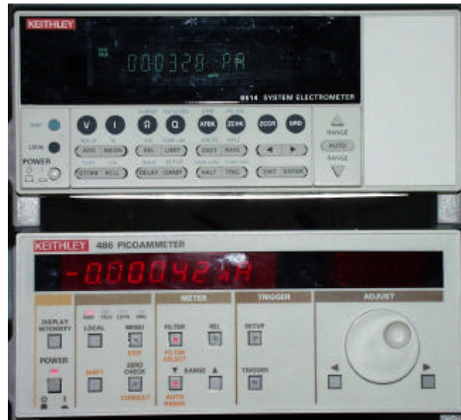
Figure 17 The two ammeters: ke486 (down) and ke6514 (up)
