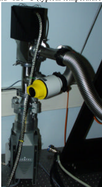
Figure 84 Testbench vacuum pump
