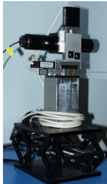
Figure 19 Motors assembly hosting a laser
