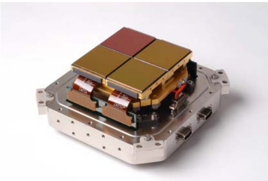
Figure 2 Mosaic of 2x2 2Kx2K Hawaii-2RG HgCdTe arrays.
